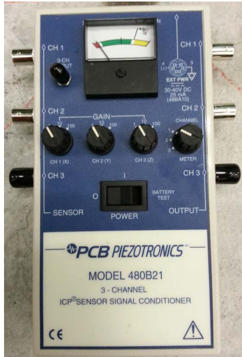
Figure 2.7. PCB model 480B21 battery-powered sensor signal conditioner.
