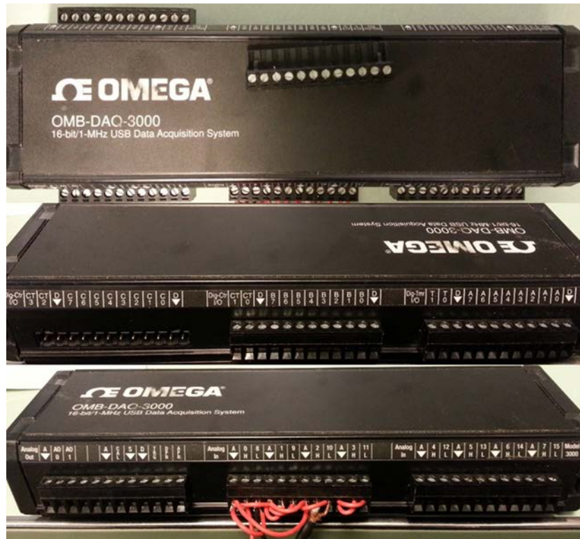
Figure 2.8. Omega OMB-DAQ-3000 1-MHz, 16-bit data acquisition system.
